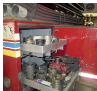
Adapters & fittings to connect hoses to the multitude of building sprinklers & standpipes.
